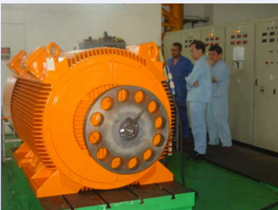
Free Load Testing at 6600V Test Bench
